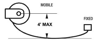
2.1.4.1 The reel is mounted on the moving object and winds up or pays out the cable as the machine approaches or moves away from the power source. Vertical Retrieve applications are possible.
