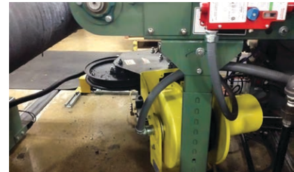
Failing cable due to the “corkscrew” effect
