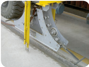
A special “wide” cable guide is used, designed to accommodate lateral movements of the RTG
