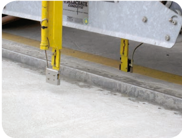
Since there are no guiding beams, two optical sensors , one on each side of the trench, control the travel deviation of the crane
